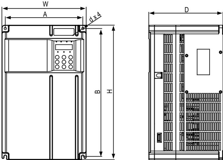
Figure 1-2 Dimension drawing of T5 to T6 models
