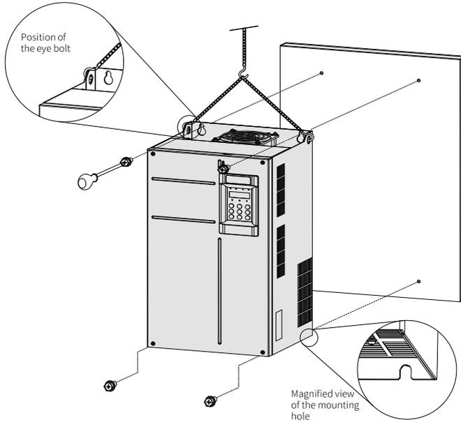
Figure 1-6 Backplate mounting (T7 to T9 models)
