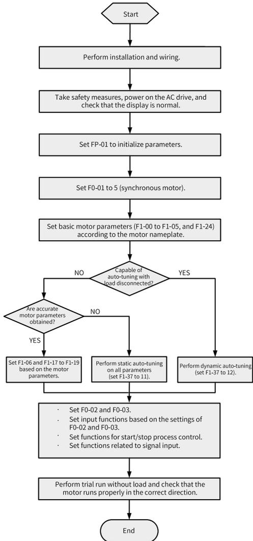
Figure 3-4 AC drive commissioning flowchart (in PMVC mode)
