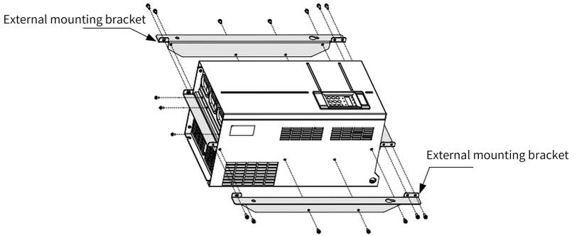
The following figure shows an AC drive with brackets mounted.
