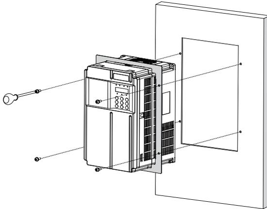
The following figure shows an AC drive that is through-hole mounted.
