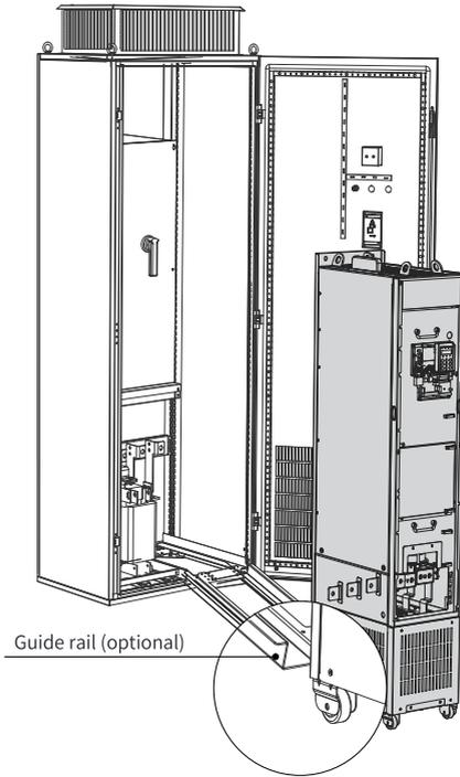
Figure 1-14 Aligning the casters with the guide rails
