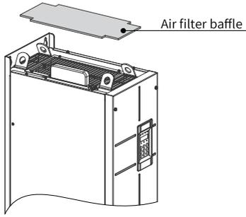
Figure 1-17 Removing the air filter baffle
