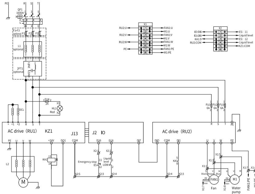
Figure 2-2 Electrical connection in a cabinet (T13 models)
