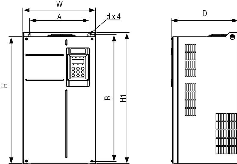
Figure 1-3 Dimension drawing of T7 to T9 models
