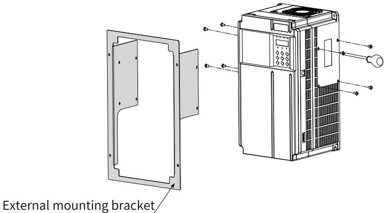
The following figure shows an AC drive with a bracket mounted.
