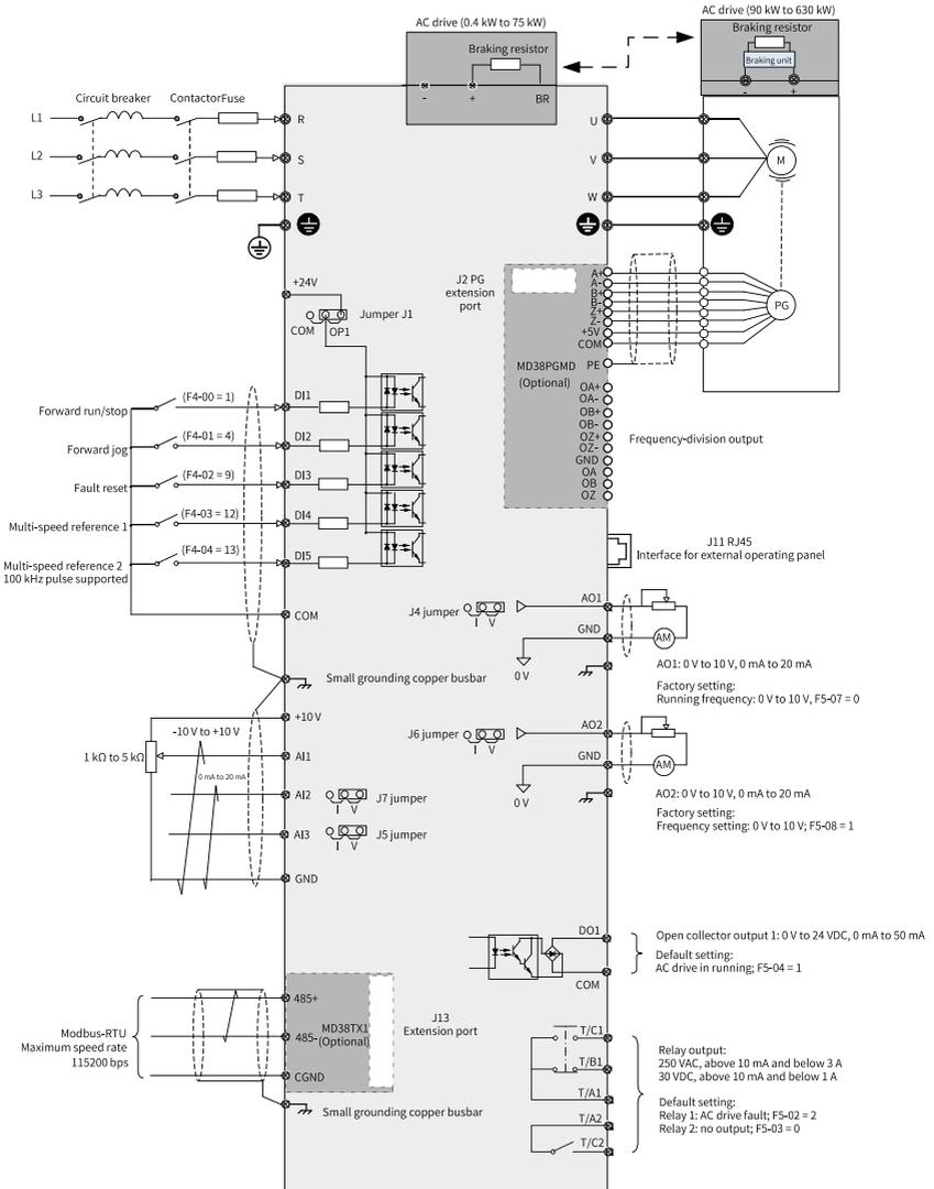
Figure 2-1 Standard wiring
