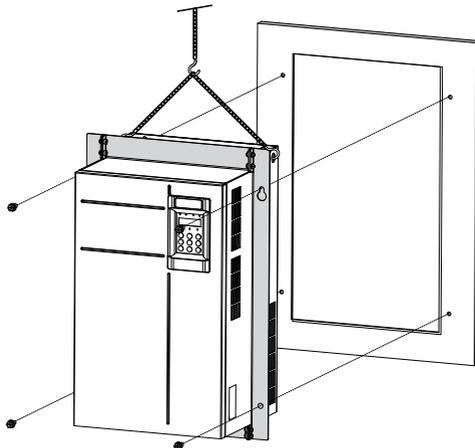
The following figure shows an AC drive that is through-hole mounted.
