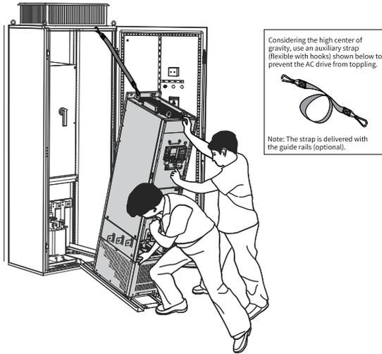
Figure 1-15 Pushing the AC drive into the cabinet
