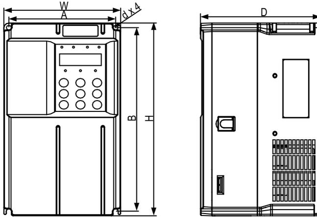
Figure 1-1 Dimension drawing of T1 to T4 models
