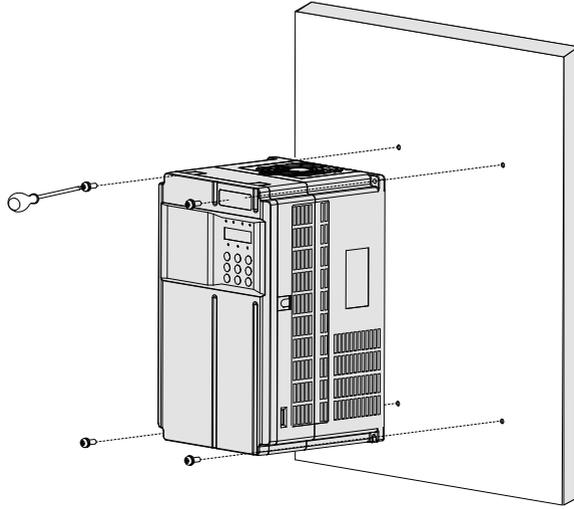
Figure 1-4 Backplate mounting (T1 to T6 models)
