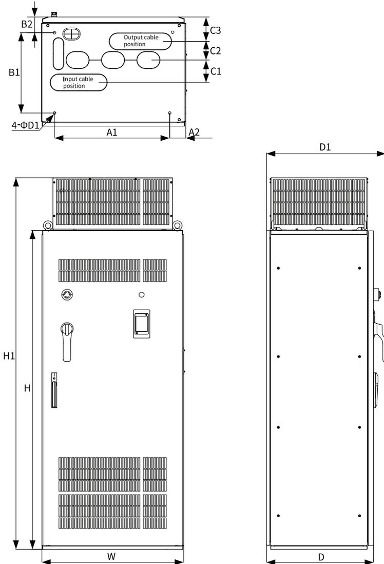
Figure 1-18 Dimension drawing of T13 models (without auxiliary power distribution cabinet)
